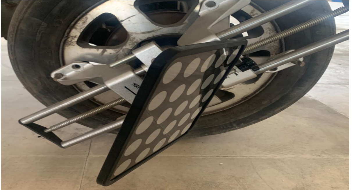
4, the target Angle is wrong or the target or the camera has gray
